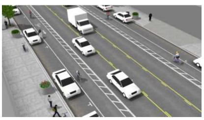
Figure 2.17 NACTO Buffered Bike Lane Example Source: NACTO Urban Street Design Guide (2013)
