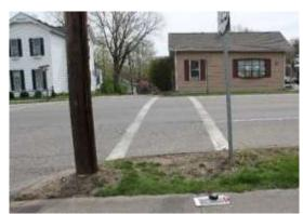
Figure 2.4 Crosswalk lacking signage and a curb ramp at West and Franklin
