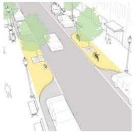
Figure 2.13 Pinch Point Source: NACTO Urban Street Design Guide (2013)
